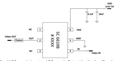
Fig. 11 DC couple Input and DC couple Output Application Circuit
