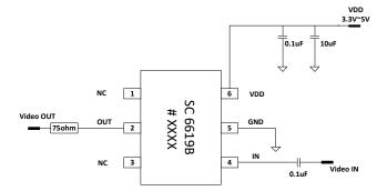
Fig. 10 AC couple Input and DC couple Output Application Circuit
