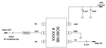
Fig. 8 AC couple Input and AC couple Output Application Circuit
