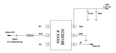
Fig. 9 DC couple Input and AC couple Output Application Circuit
