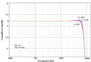
Fig.3 Cload Variation For Gain Vs Frequency
