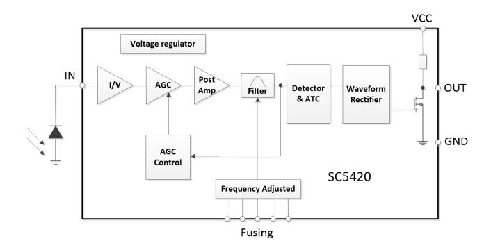
Fig.1 block diagram of SC5420
