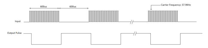
Fig.2 The output pulse of 37.9 KHz carrier frequency with 22 pulses burst
