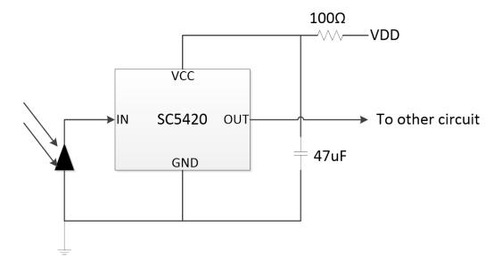
Fig.2 Applications Circuits of SC5420
