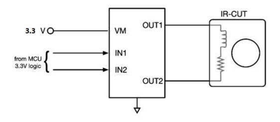
Figure 2. Schematic of SC8891 Application
