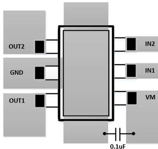
Figure 4. Simplified Layout Example
